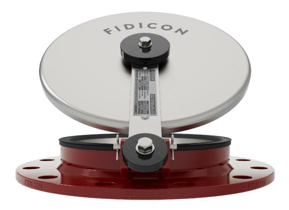
As emergency venting device for installation on storage tanks with a VRV to protect against hazardous excess pressure but minimize the loss of gas/vapours. also suitable as replacement of a manhole. it does not protect against the hazard of explosion or stabilized burning,
