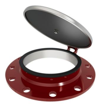
It is designed to relief particularly large amounts to prevent the vessel from rupturing in an emergency case. Device will start to open as soon as the set pressure is reached and requires only 10% overpressure for full lift.
